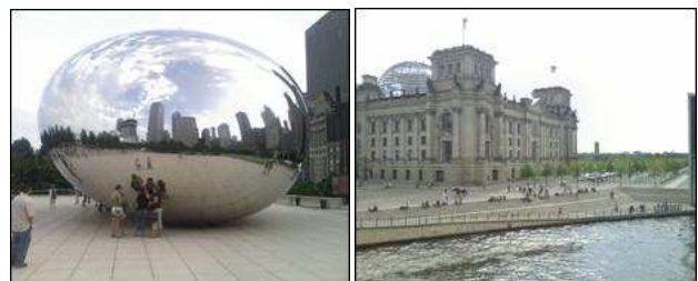
Fig. 1 Examples of frames from image sequences captured with a typical camera phone. Notice the absence of any information in the sky. This is due to the limited dynamic range of the camera module.
