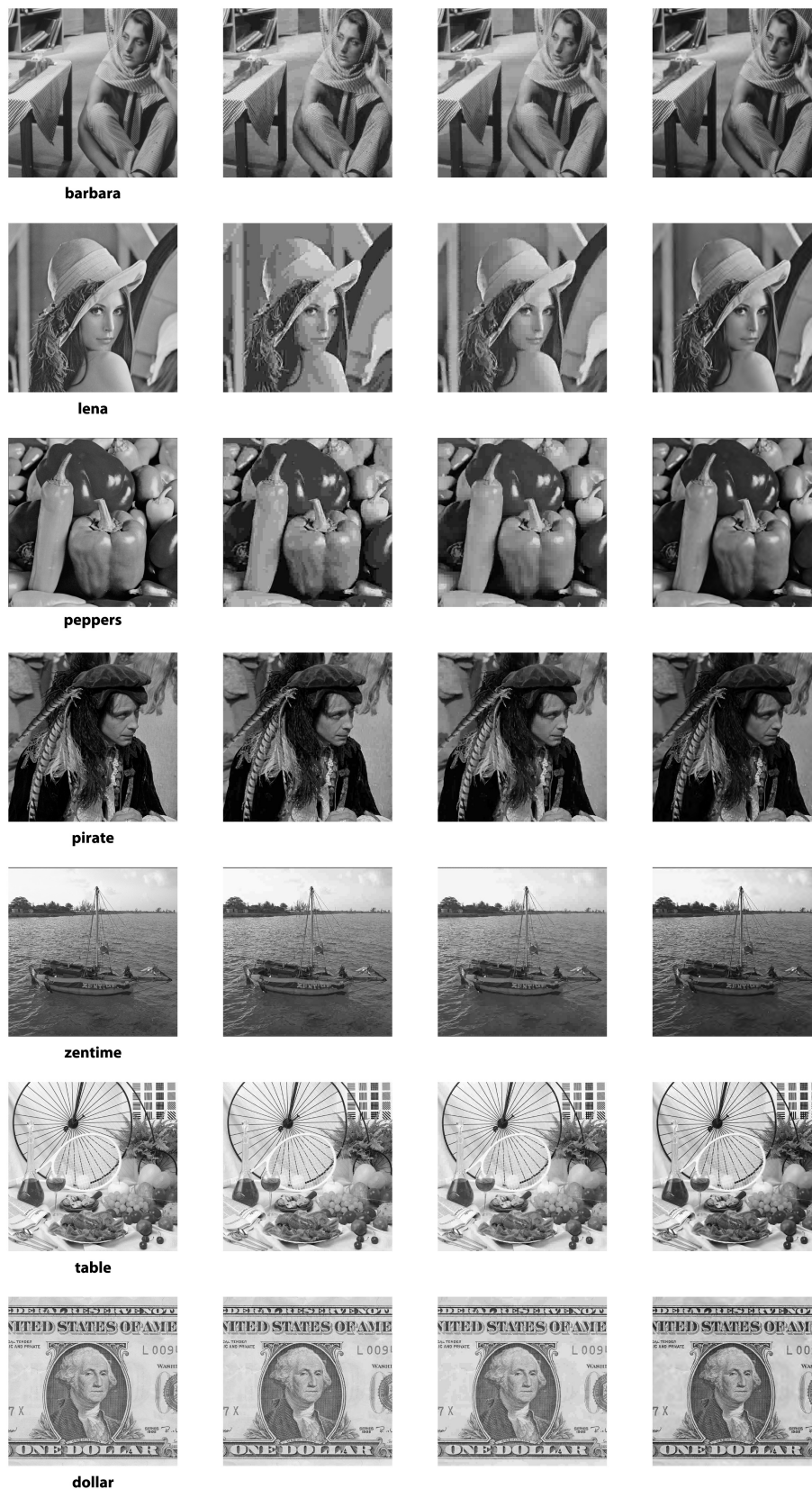
Figure 5.5: Visual comparison of the schemes (medium bit-rate). Left to right: Original, JPEG, Sparse K-SVD and JPEG2000.
