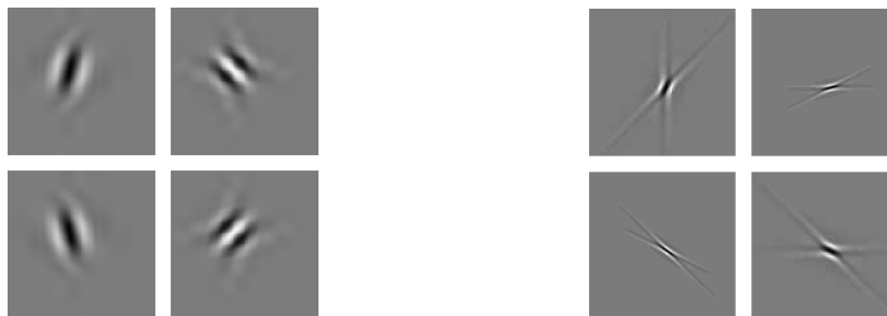
Figure 3.6: Left: a few complex wavelet atoms (real part). Right: a few shearlets.
