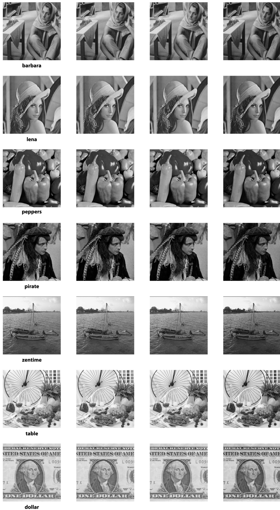
Figure 5.6: Visual comparison of the schemes (high bit-rate). Left to right: Original, JPEG, Sparse K-SVD and JPEG2000.
