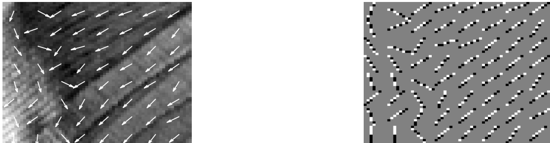
Figure 3.5: Left: the flow in a specific image region. Right: some bandelet atoms adapted to the region. Note how the 1-D wavelets are skewed to follow edges.
