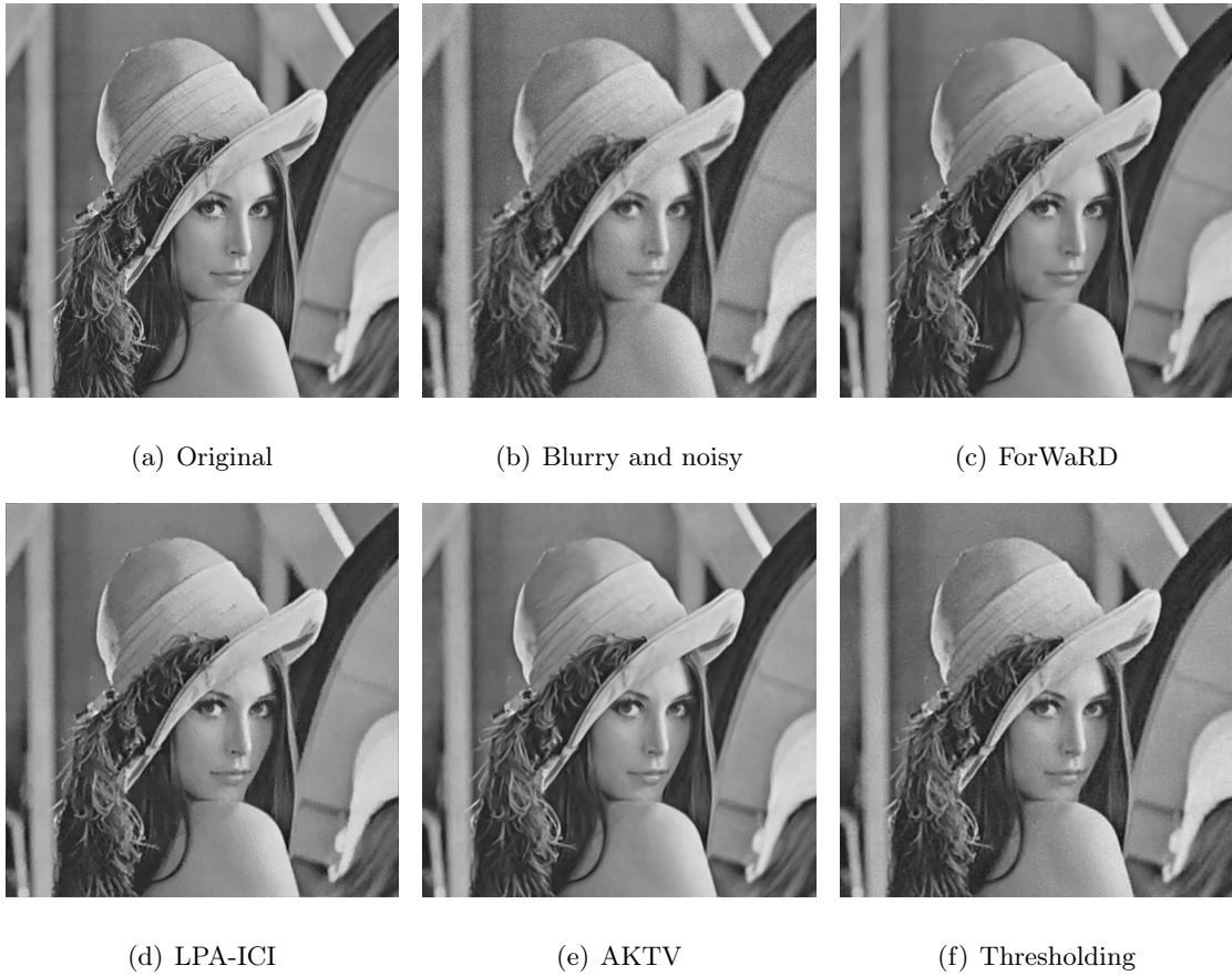
Figure 7.4: Deblurring results for Lena . Blurring kernel is a 5 \times 5 Gaussian with standard deviation 1.5, additive noise is white Gaussian with standard deviation 8.25 (BSNR=15dB). RMSE values are 10.78 (blurry), 7.55 (ForWaRD), 6.76 (LPA-ICI), 6.12 (AKTV) and 6.69 (Thresholding). Thresholding parameters: block size is 10 \times 10 , dictionary size is 256 \times 100 .
