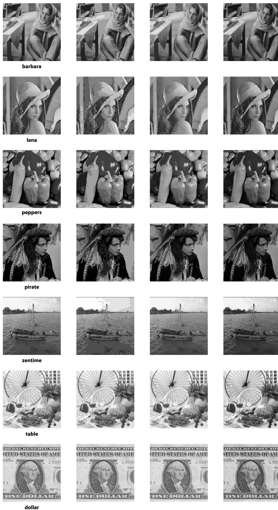
Figure 5.4: Visual comparison of the schemes (low bit-rate). Left to right: Original, JPEG, Sparse K-SVD and JPEG2000. For the images Lena and Peppers , where JPEG could not achieve the target file size, the shown images use the lowest possible quality settings.
