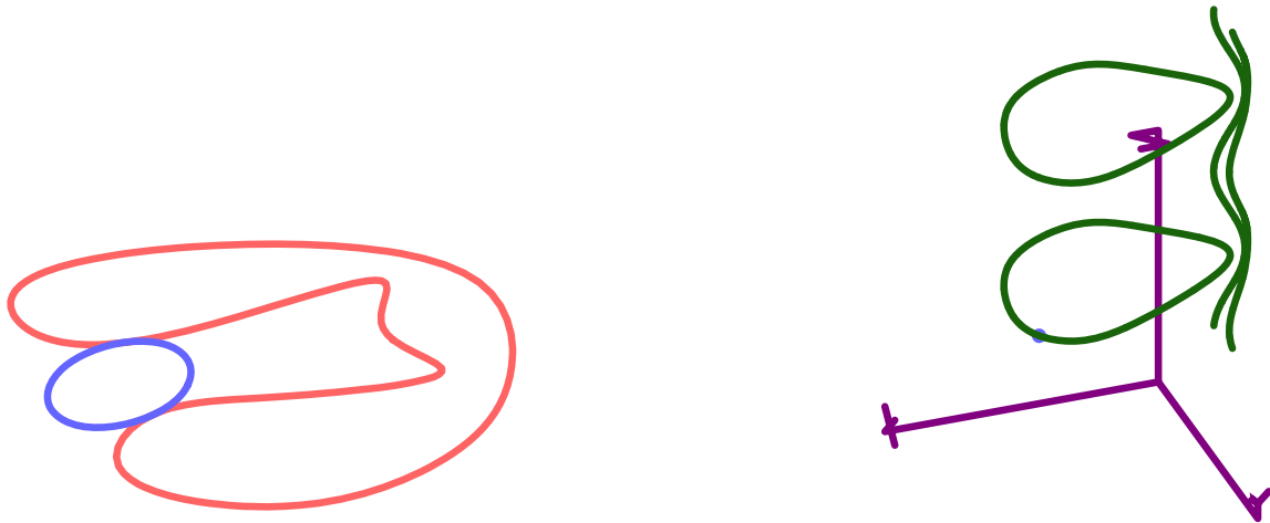
Figure 12: The precise configuration space (three axes for the three degrees of freedom - XY motion and rotation in the plane) is shown on the right for the two curves on the left. The specific configuration on the left is designated as a point on the right. Computed by mapping the contacts formulation into algebraic constraints and solving them.
