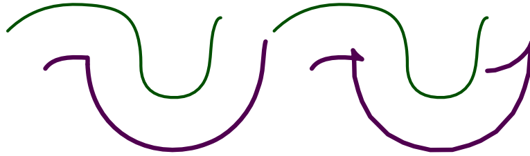
Figure 5: Adaptive offset approximation (thick) of a B-spline curve (thin). On the left, the self intersections in the offset computed in the right are eliminated. Both offsets were computed using AOFFSET. (See also Figure 77.)
