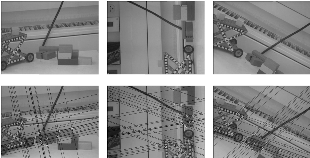
Fig. 9. (Top) Three images of a scene. (Bottom) Fifteen triplets of corresponding points have been extracted and the points (denoted by the circles) and their respective epipolar lines have been overlaid over the original images.
