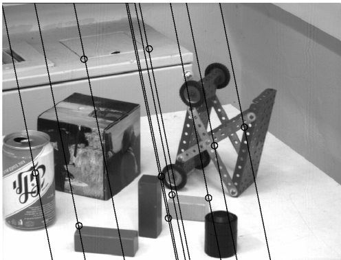
Fig. 2. Two images of a scene. Ten pairs of corresponding points have been extracted and the points (denoted by the circles) and their respective epipolar lines have been overlaid over the original images.
