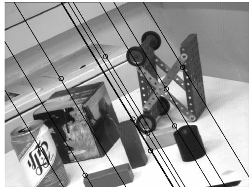
Fig. 2. Two images of a scene. Ten pairs of corresponding points have been extracted and the points (denoted by the circles) and their respective epipolar lines have been overlaid over the original images.
