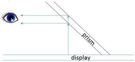
The first prototype was I built was small, and made out of CD-ROM cases. The CD-ROM case was thinner than the perspex of the final prism, thus creating a sharper image.
